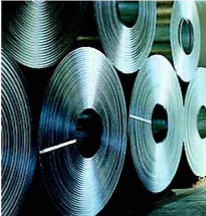
ArcelorMittal, the largest steel corporation in the world, recently looked for a safe and reliable automation solution for transporting steel coils at their flat carbon steel products plant in Ghent, Belgium. Coils, which can weigh 30 tons, first need to be lifted safely and securely from incoming rail wagons and then be placed on 'saddles' in the stockyard (a temporary storage area). Later, they are picked up and delivered 'just in time' to the right
